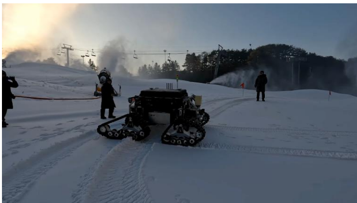
Figure 2: Robot testing in low-temperature environment. (Credit: KOPRI)
