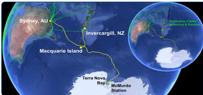
Figure 3: Proposed Antarctic subsea cable routes: McMurdo Station to either Sydney, Australia or Invercargill, New Zealand. (Credit: USAP)
