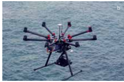
Figure 1: Two extremes (a) A $US400,000 Schiebel CAMCOPTER S-100, used by the French, Brazilian, and Italian Navies, capable of autonomous missions of 10 hours endurance with 30 kg payloads, 200 km from its point of origin (b) An octocopter (DJI S1000) of the type used on the RV Nathaniel B. Palmer voyage in 2015. Approximate cost is $AU10,000 with an estimated endurance of 20 minutes, payload dependent.
