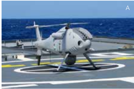
Figure 1: Two extremes (a) A $US400,000 Schiebel CAMCOPTER S-100, used by the French, Brazilian, and Italian Navies, capable of autonomous missions of 10 hours endurance with 30 kg payloads, 200 km from its point of origin (b) An octocopter (DJI S1000) of the type used on the RV Nathaniel B. Palmer voyage in 2015. Approximate cost is $AU10,000 with an estimated endurance of 20 minutes, payload dependent.
