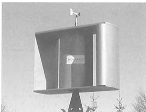
Figure 1 – The turbine of the vertical axis wind generator. Note the anemometer on the top.
