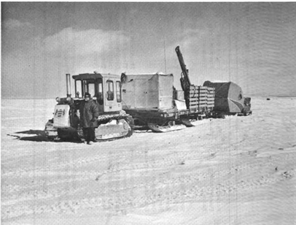
Figure 2. D4 caterpillar tractor hauling seismic drill cab, living caravan and fuel.
