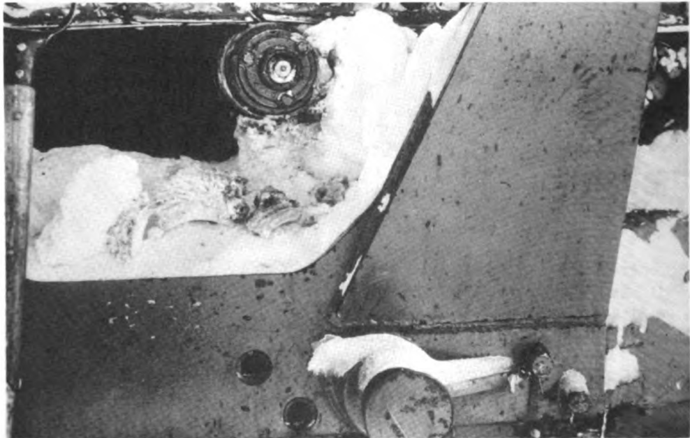
Hard ice build-up on track support roller 1958.
