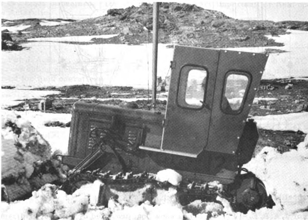
Figure 14. The feature of an angle-dozer modified to cabin type.
