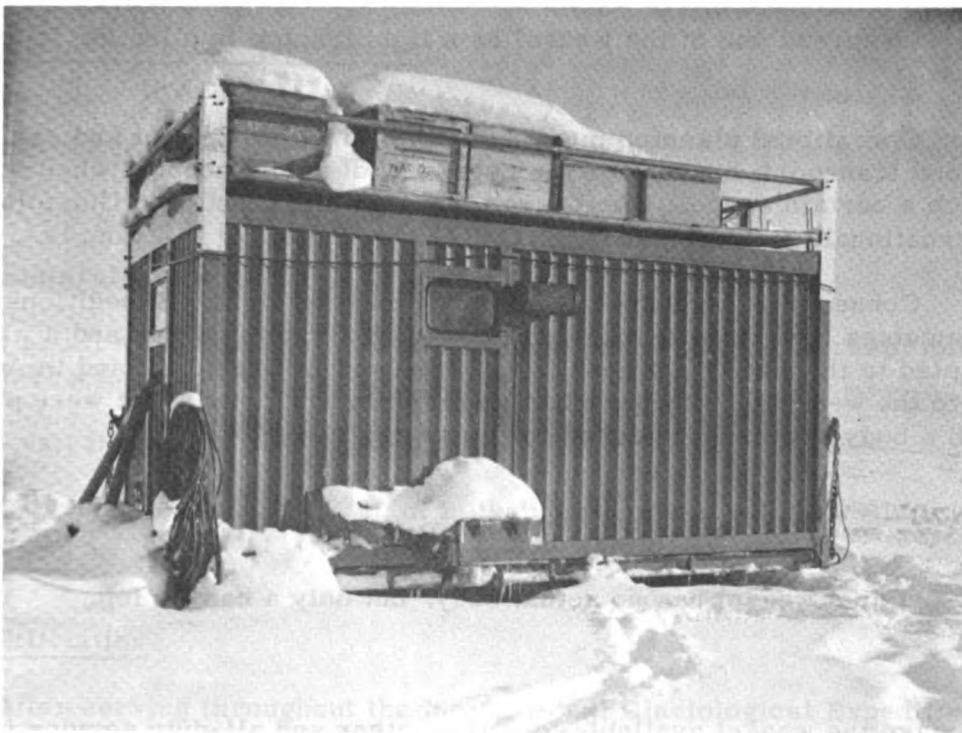
An A. N. A. R. E. Sledge-Mounted Caravan with Stores Rack Fitted to the Roof.
