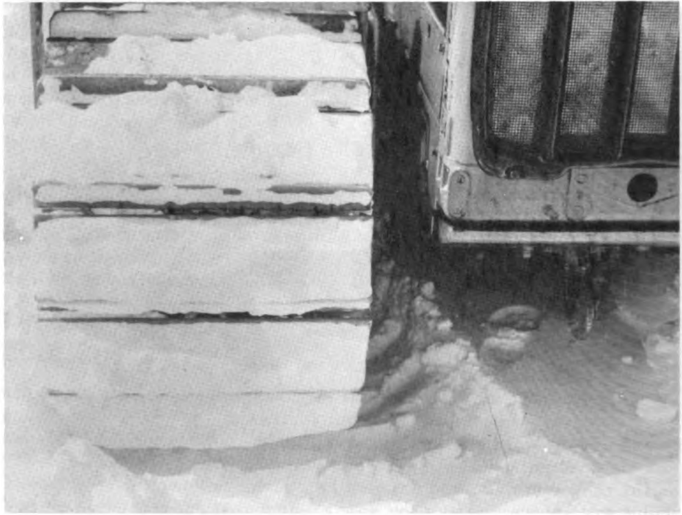
Soft snow compacted on track plates 1960.
