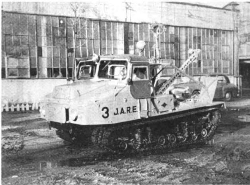
Figure 4. The feature of Komatsu "Ginrei" Model KC20-3R gasoline snow-wrecker.
