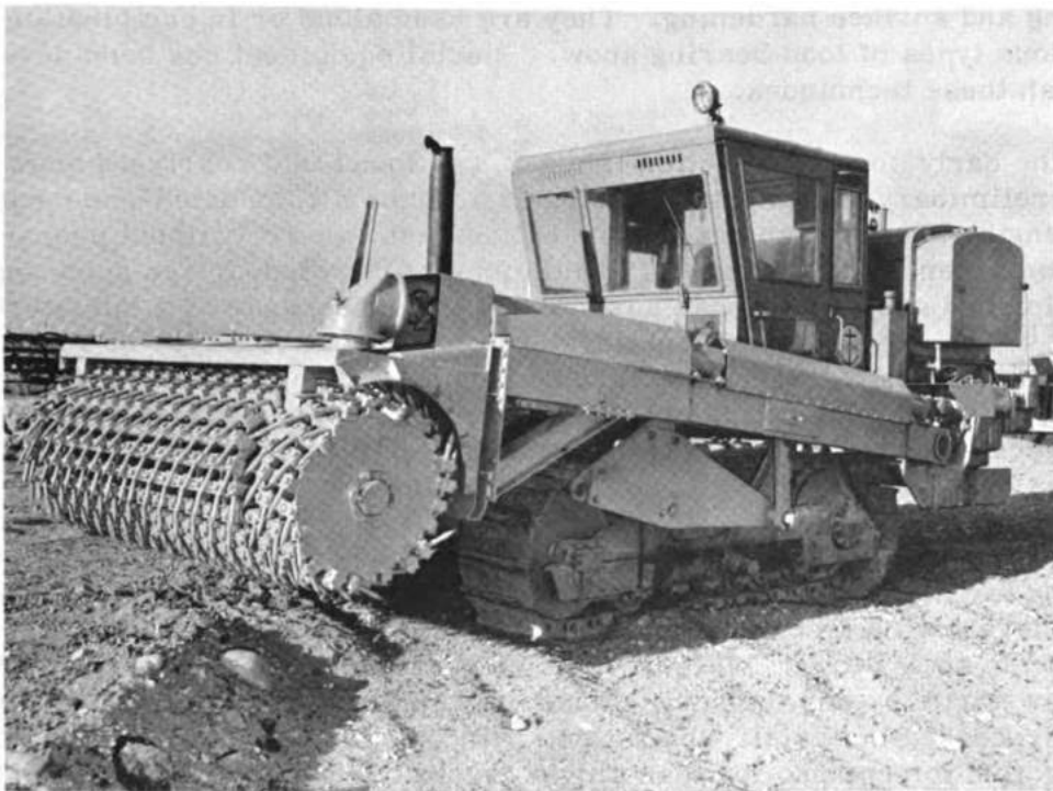
Figure 4. Ice cutting drum on the ice dozer.
