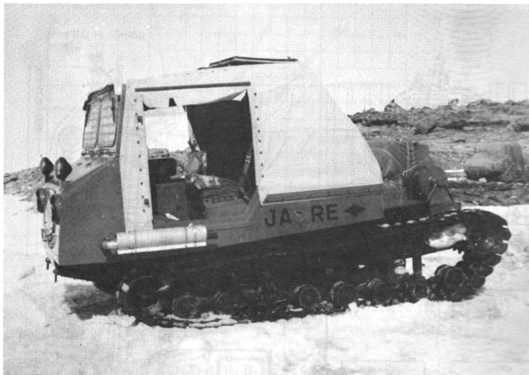
Figure 11. The feature of KD 20-2T cab-over type diesel snow-car at the Syowa Base.
