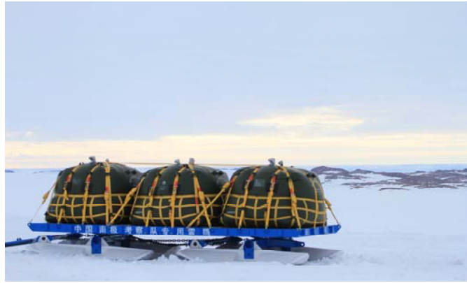
Figure 4: During the inland transport, three flexible tanks were fixed on each sled, equivalent to 75 drums
