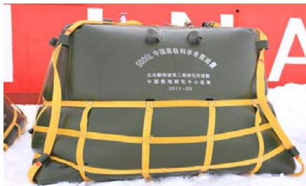
Figure 2: The shape of the full flexible tank
