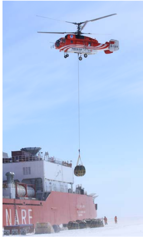
Figure 3: Lifting the 5000 L flexible tank by the helicopter
