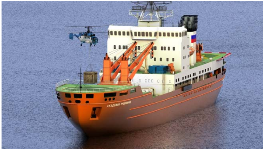
Figure 1: A computer-generated model showing the proposed design of the new vessel Akademik Tryoshnikov
